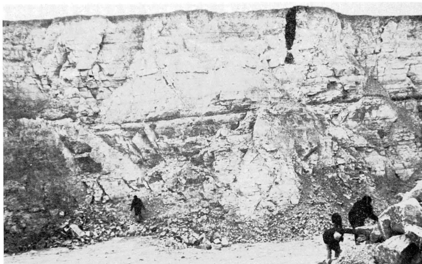
Plate 8. Tetford Hill Chalk quarry with Pink Band (dark line across centre) and solution pipe (?) at surface. (TF 329760) (Photo by D. N. Robinson)
